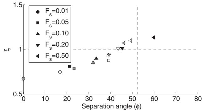
FIG. 17. Relation between separation angle and overall drag value ( $Re = 100$ ,  $h/b = 0.1$ ). White symbols:  $n_b = 1$ , grey:  $n_b = 3$ , black:  $n_b = 7$ . The dashed line is for a no-slip sphere.<sup>20</sup>
